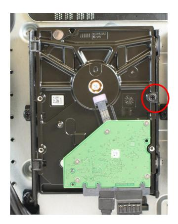
4. Remove the hard drives from the bracket.
