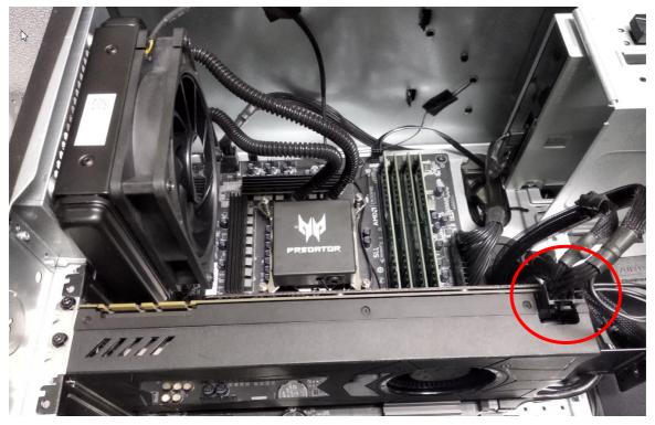
3. Remove the screw that secure the Graphic boards to the chassis.
