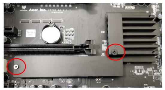
4. Remove the thermal heat-sink module from the mainboard.
