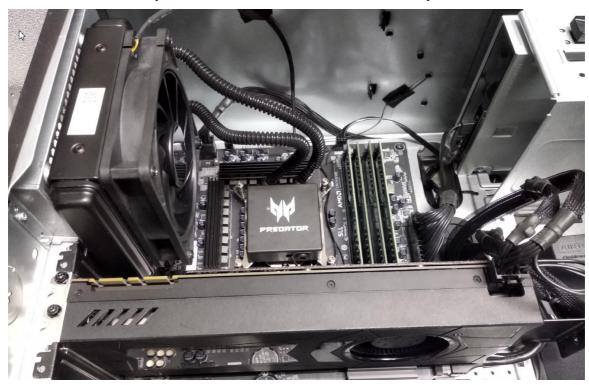
4. Connect the power cables to the Graphic boards.
