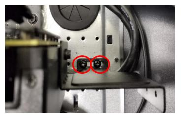
4. Release the latch that secures the graphic board to the mainboard.
